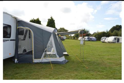
To attach the draught skirt; insert the beading into the bottom awning channel on the vehicle and slide to the desired position.
