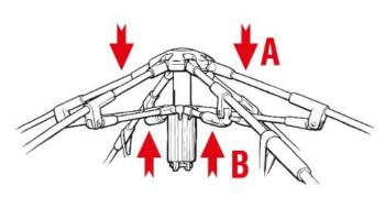
Fold each leg into the middle central hub ensuring it is as compact as posisble to repack into the bag. NOTE – FOR THE LEGS TO FOLD ALL HINGES MUST BE IN THE UN-LOCKED POSITION. DO NOT APPLY EXCESS FORCE AND THIS MAY CAUSE DAMAGE TO THE FRAME.
