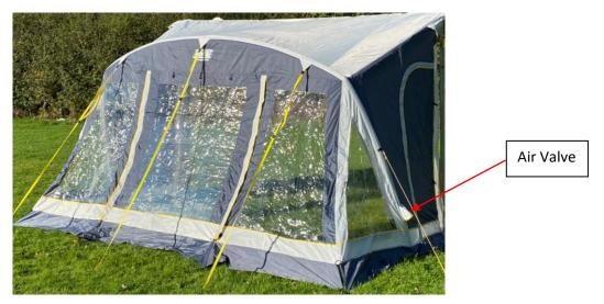
Connect the large adaptor to the hand pump. Insert the adaptor into the top cap on the valve. Inflate the air beam to approx.6-7 PSI. Once inflated; remove the adaptor from the valve and securely tighten the top cap. WARNING: WHEN INFLATING; DO NOT EXCEED A PRESSURE OF OVER 7 PSI. IN STRONG SUNLIGHT & IN HOT TEMPERATURES REDUCE THE PRESSURE TO 4-5 PSI.
