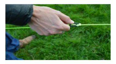
It is recommended each peg is driven fully into the ground at an angle of 45 Degrees away from the pegging point.
