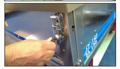
Ensure all fixings are secure, and all persons are clear before releasing the ABS cover.
