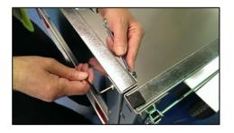
1) Remove the Hex bolts found at the top of the front panel corner posts (2x M8) and rear panel (2x M6) near to the sides, and replace with the corresponding supplied cap-head screws using a hexagonal key and the original nyloc nuts.
