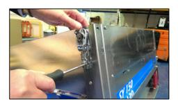
2) Fit the overcentre catches to the sides of the trailer at the rear, using the two lower holes of the groups of three in the trailer corner posts, using the supplied coutersunk screws and M5 locking nuts. Fully tighten the nuts with a spanner.
