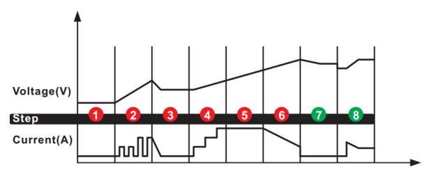
**Stage 1** — Diagnosis: The battery is analysed to ensure it can be charged, so as to prevent charging a defective battery.
