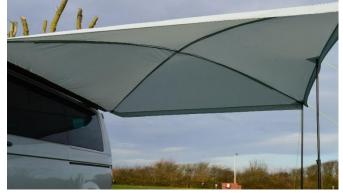
Adjust the height of each leg to suit the ground level to achieve a level height. It is recommended the height of each leg should be approximately the same level as the awning channel on the vehicle. Adjustment can be made by using the leg pole adjuster as shown below:
