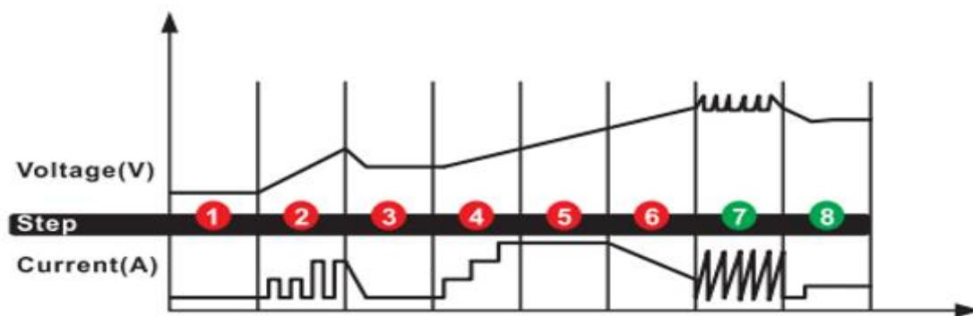
**Stage 1** — Diagnosis: The battery is analysed to ensure it can be charged, to prevent charging a defective battery.
